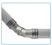
In the renovation business very often the buildings are old fashioned and the rooms are not at right-angled. In big dimensions it is not possible to bend the pipe with a small bending radius. The short spacers RS 2 and RS 3 allow you to combine two elbows 45° to an elbow for the angle you need. They are also useable for the outlets in the riser pipe to cross them with the shortest possible distance.
